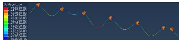
Fig. 7 Deflection of the beam under finite element simulation
