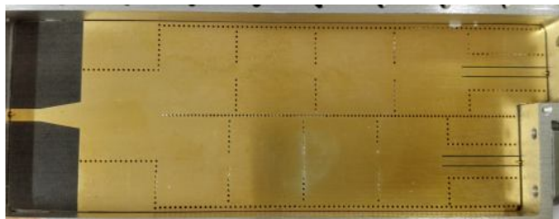
Fig. 7 Photograph of the fabricated diplexer
