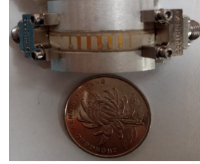
Fig. 9 Photograph of the fabricated conformal filter
